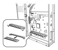
5 Insert the new DIMM straight down into the DIMM connector until the latches snap into the locked position.
